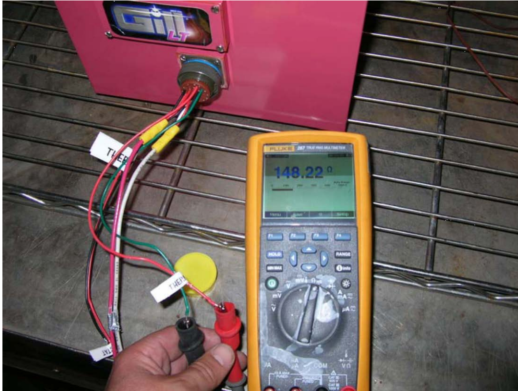
Figure 6: Verification of Heater Blanket Connection – Pins MNP–RSF
